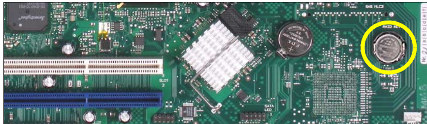
Figure 28: Inserting the RAID key
