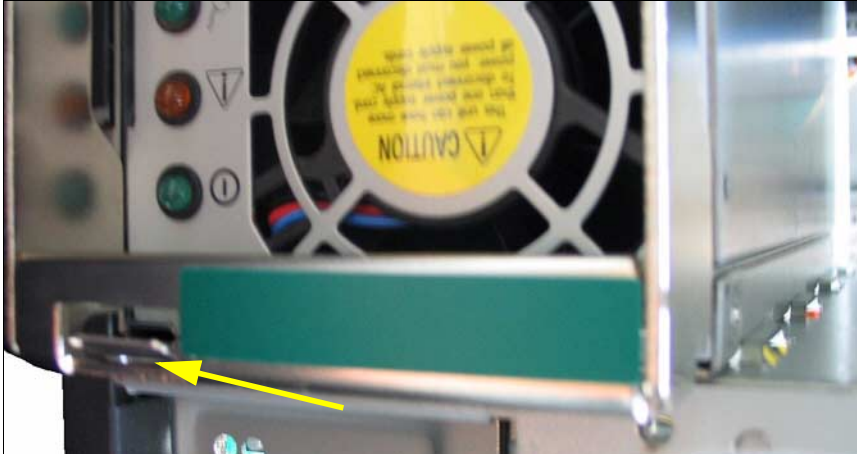
Figure 41: Locking the power supply module
