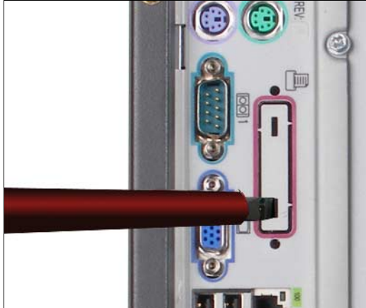
Figure 31: Breaking off the interface plate
