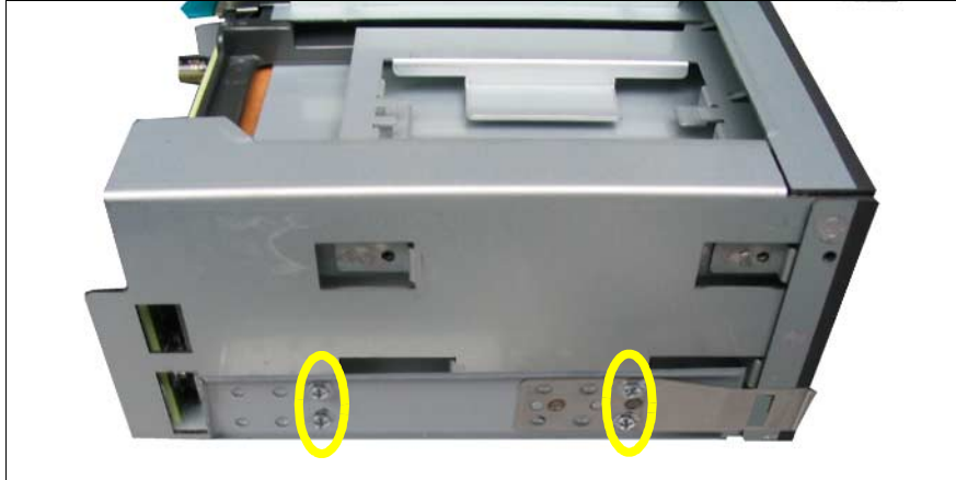
Figure 23: Attaching the EasyClick rails
