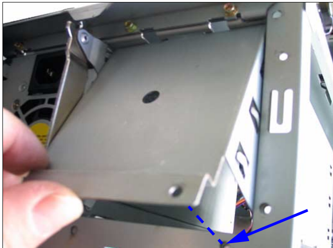
Figure 42: Installing the dummy cover
