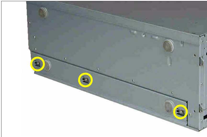
Figure 48: Removing the rubber feet
