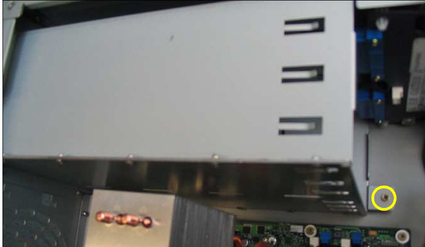
Figure 38: Fastening the PS cage in the housing
