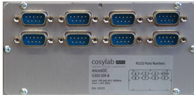
Figure 15: example of back-panel connectors (8 COM ports, desktop 2U case)
