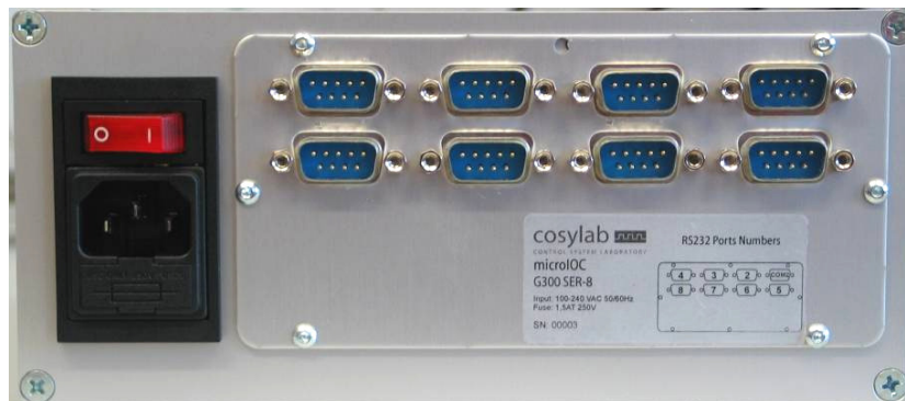
Figure 9: back panel of the desktop 2U case microIOC, showing mains connector and extension connectors
