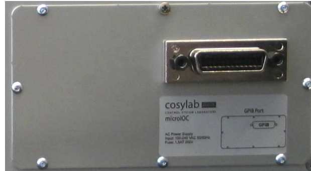
Figure 18: example of back-panel GPIB connector (desktop 2U case)
