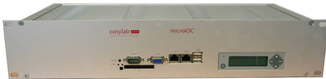
Figure 1: customizable and reliable remote control for various end-point devices (desktop 2U case with LCD)
