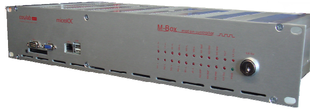
Figure 22: customized front panel of M-Box motion controller
