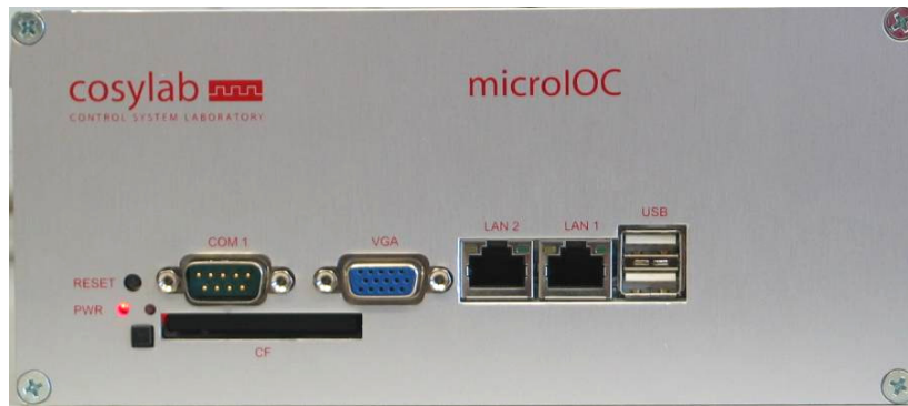
Figure 8: front panel of the desktop 2U case microIOC unit
