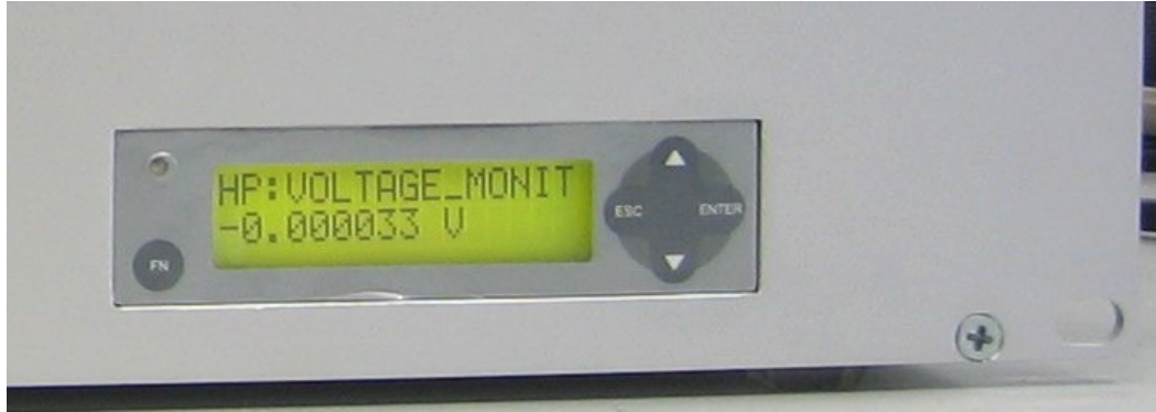
Figure 11: LCD display mounted into rackmount case and displaying voltage measured by HP multi-meter (connected via microIOC's GPIB port)
