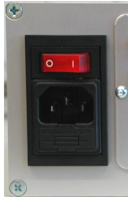
Figure 10: IEC mains connector with fuse and switch with indicator light
