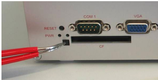
Figure 5: extracting CF card, step 1
