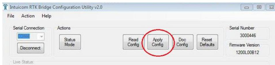
**Figure 16: "Apply Config" Loads the Configuration onto the RTK Bridge-C**
