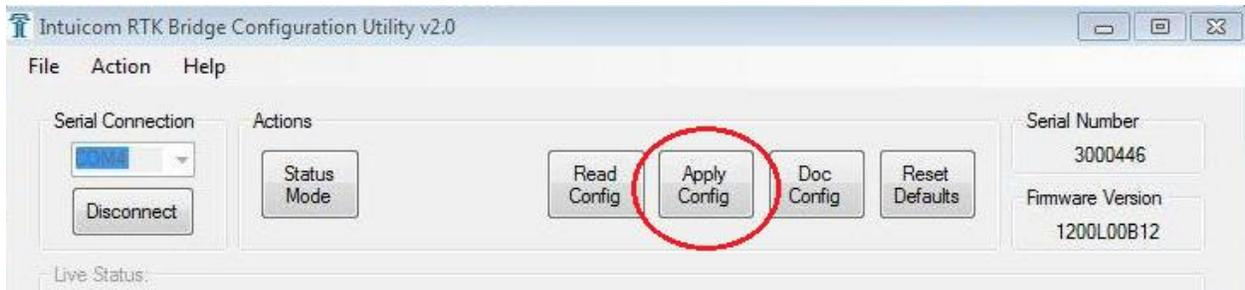
**Figure 10: Apply Configuration” Loads the Configuration onto the RTK Bridge-C**
