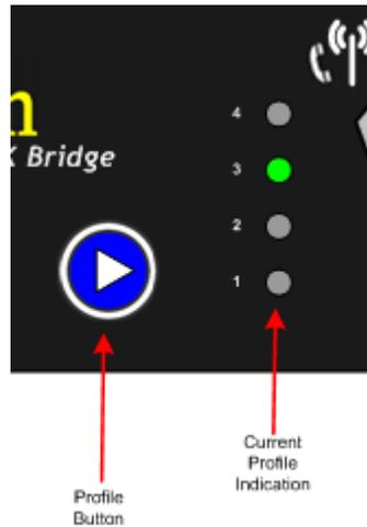
**Figure 23: Changing the active profile on the front panel**
