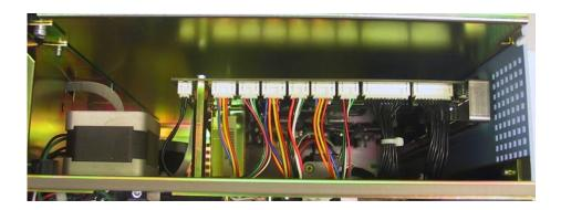
The mono electronic board is located between the hydraulic part and the reagent tray.
