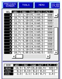
This screen allows carrying out a test of repeatability on all the parameters measured by the MYTHIC 18.
