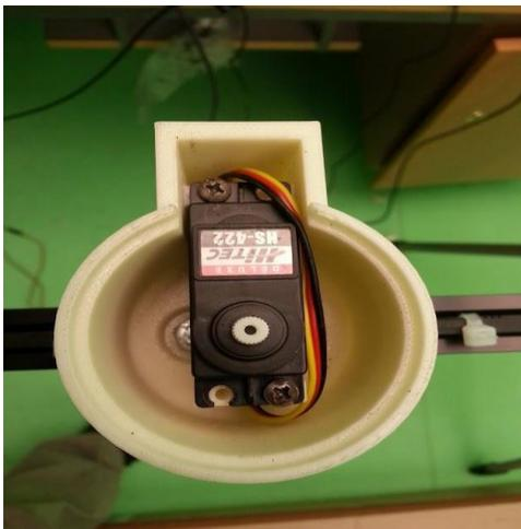
Figure 53: 3D-printed casing with the pan-servo
