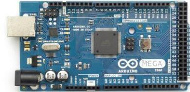
Figure 59: Arduino Mega 2560
