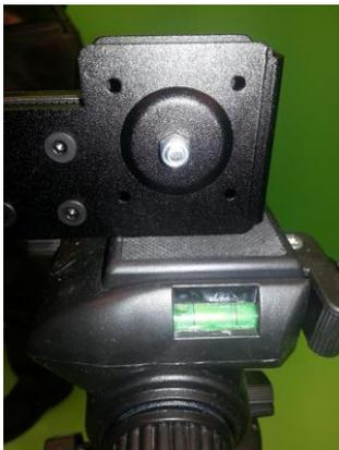
*Figure 55: The tripod is connected to the rig endmount*
