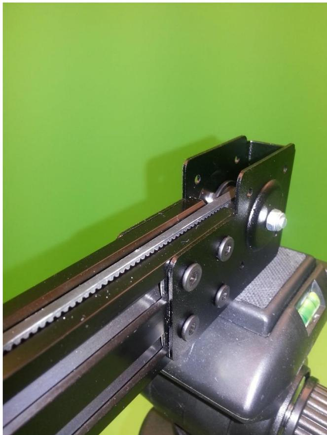
Figure 42: The End Mounts on the rail
