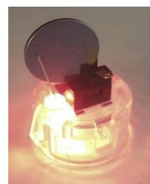
Figure 63: Arcade Button with custom LED
