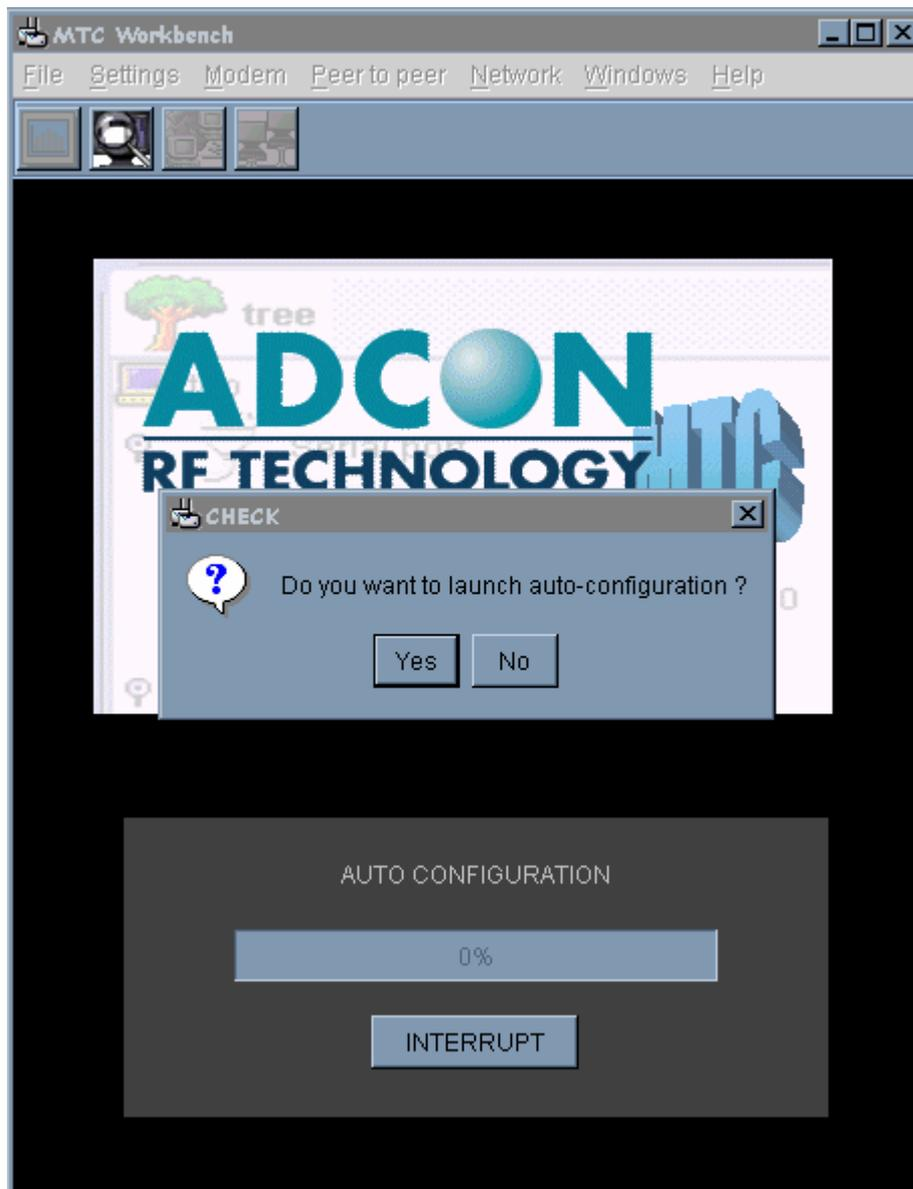
The auto-configuration has to be launched for the software to detect the connected radio module, i.e. 'Yes' has to be pressed.
