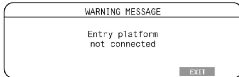
Check the load bar connections to the Scale.
