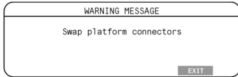
The load bars are connected to the Scale in the wrong order. Swap them around at the Scale.
