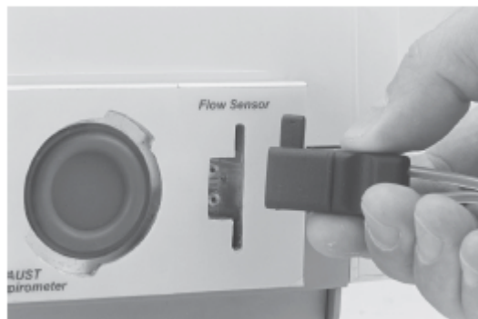
Figure 4.1 - Detail of the flow sensors connection on the side panel of an Inter® Plus system ventilator.
