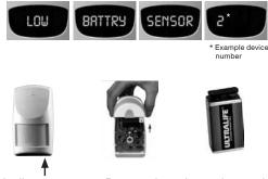
Unclip cover at the bottom. Remove the cover. battery.
