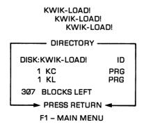
The number in front of the filename refers to the number of blocks used by that file. The last column shows what type of file it is (see the disk drive manual for more details).
