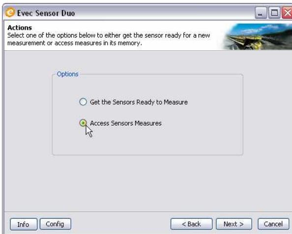
**Figure 64: Accessing Sensor Measures**
