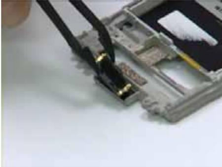
2. Attach the receiver to Chassis.
