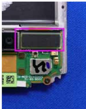
10. Disconnect the FPC connector from the Upper board.
