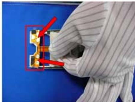
5. Remove the release paper and stick AP key FPC on the Chassis as shown
