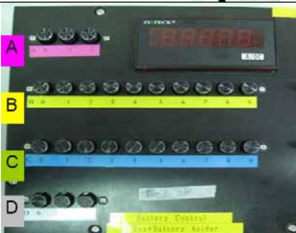
Set up each button by row A~D according to product specification Following is an example for Sapphire
