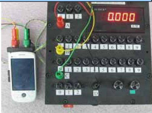
Power off the device and measure the sleep mode current.
