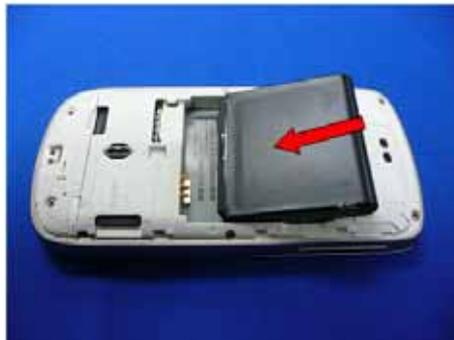
26. Insert battery into housing.
