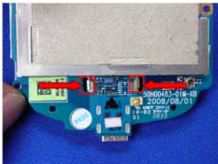
3. Insert the switch hook into the Main Board
