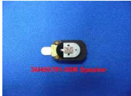
6. Disassemble speaker from keyboard bottom cover.
