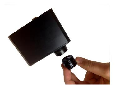
Be careful when you replace the infrared lens. The lens has a delicate anti-reflective coating.
