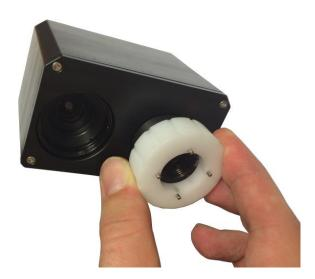
In order to focus on short distance gently rotate the lens counterclocwise. During this movement, the lens extends from the camera body. If the lens can rotate too easily, you probably get on the edge of the focus range. Trying to rotate the lens more may cause the lens to fall out.
