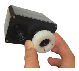
2) Perform lens replacement pointing the lens pointing downwards. This prevents the dirt settlement on infrared chip. Never point infrared camera without lens to any light source.
