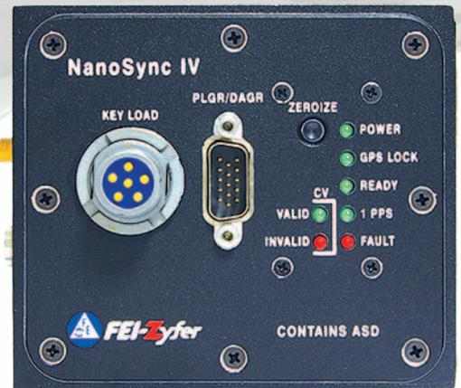
Status LEDs, Key Load Port, PLGR/DAGR Port & Zeroize switch
