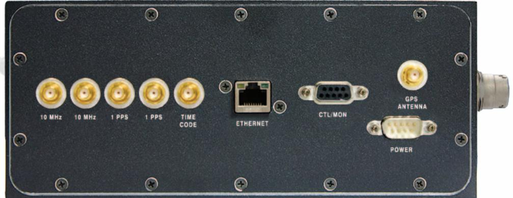
The NanoSync IV is a small form factor GPS Position, Navigation, Time (PNT) and Frequency reference system that provides multiple reference outputs and includes support for NTP & PTPv2 IEEE 1588-2008. The NanoSync IV has a Rubidium oscillator and is equipped with a SAASM receiver (Rockwell-Collins MPE-S GB-GRAM or Trimble Force 22E MRU) for military users. The NanoSync IV is packaged in a small, rugged enclosure ideally suited for embedded electronic warfare applications.
