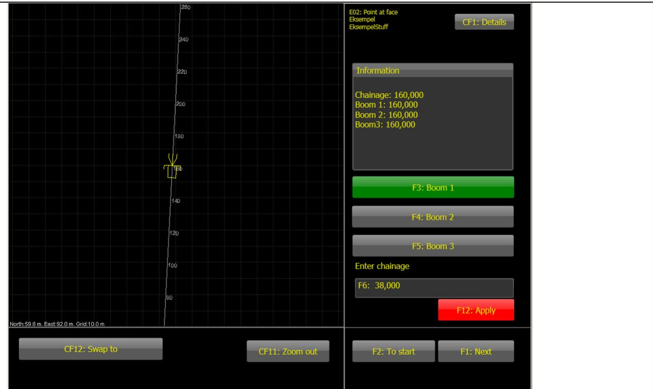
When the drill rig is navigated it is still necessary to define the position of the face. The face is a vertical plane perpendicular to the tunnel line. It is used as reference for measuring of the hole depths when hole depth is not measured from collaring position. The chainage value for the face is the reference for the position of the log for the round. The face can be pointed out with a boom or by typing a value.
