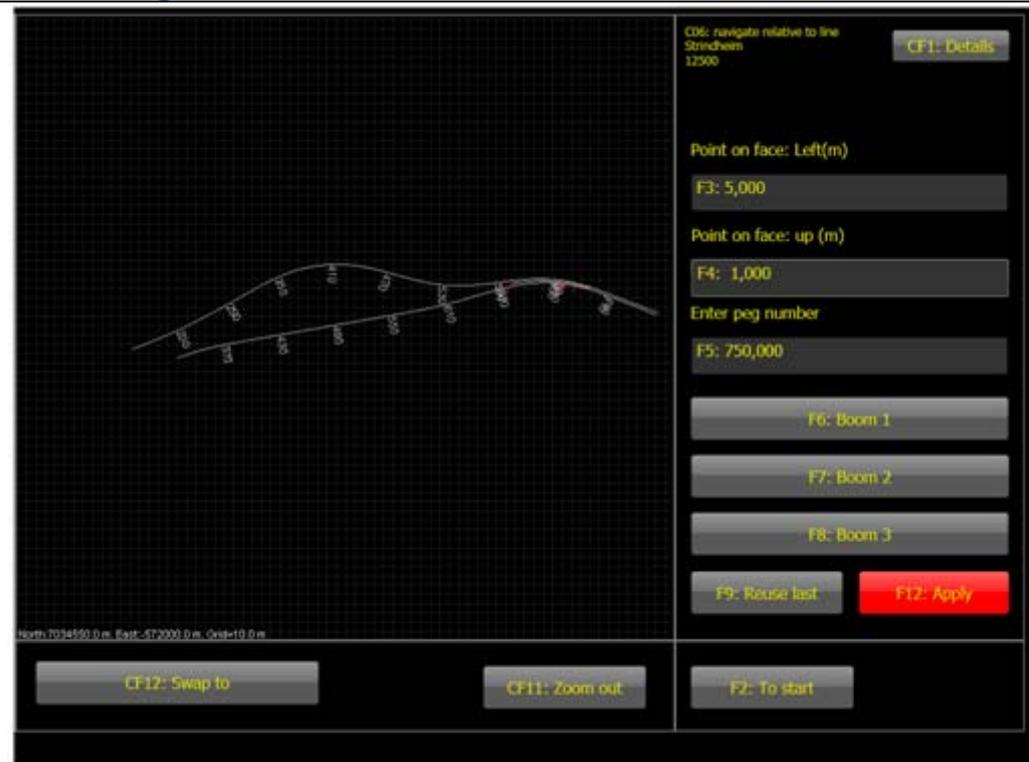
This is a simplified laser navigation and normally used in mines only. One of the booms is positioned on a mark or known position on the face with the feeder in level. Then the distance sideways and in height with respect to the centre of the floor are typed into field F3: and F4:.
