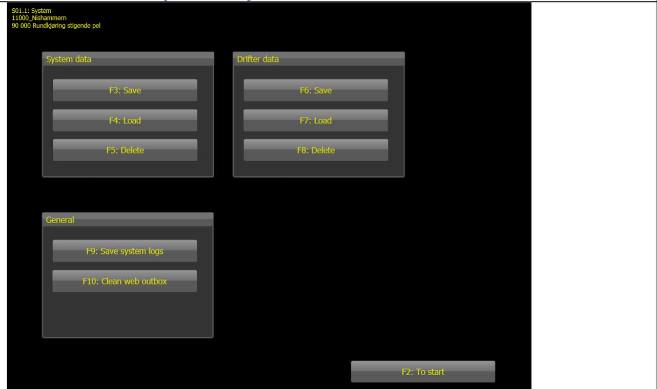
This menu is for saving and restoring system data and drill parameters to and from the hard drive of the computer and a USB memory stick. System data are parameters like geometry parameters, scaling factors, calibration values and so on. Drifter data are drill parameter settings for the different drill parameter sets.
