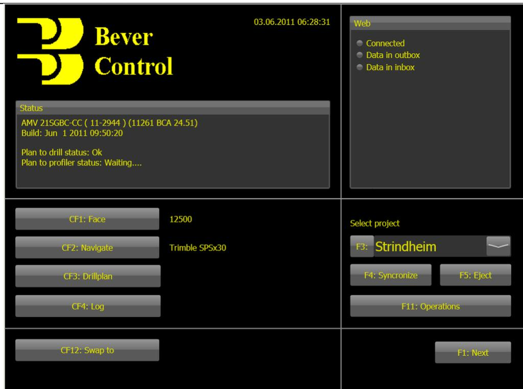
This menu is the start menu and main menu for BeverPlan, and can always be reached by pressing F2:To start. The status information shows if the program is connected to the BeverDrill and BeverProfiler programs.
