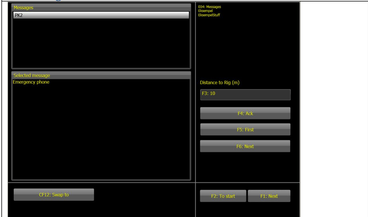
It is possible to send messages from the office to the drill rig operator. The message is printed on the screen when the drill rig is inside the radius in F3:Distance to rig. The centre of the radius is the fixed point connected to the message. Example of messages are information of emergency stop telephone niche, pump station and other installations not shown in the contour or drill pattern.
