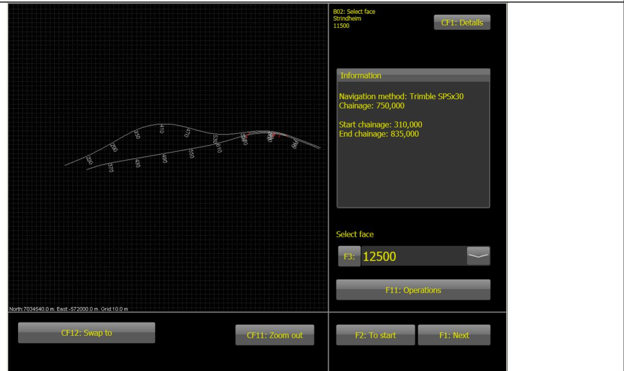
In the office a face is defined with name, drill direction, tunnel line and drill patterns. On the drill rig data like navigation method, current chainage value and last used drill pattern are saved for each face.
