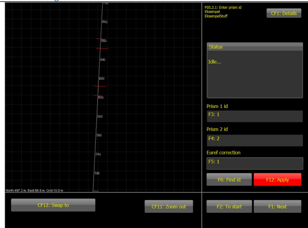
This menu is used to test a prism if the total system has problems with detecting it and to set some parameters.
