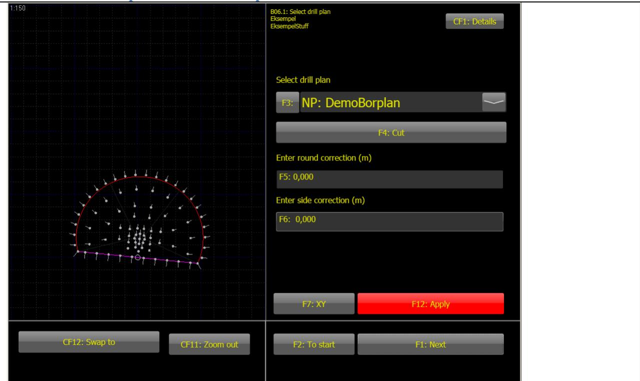
It's recommended to make separate drill plans for round, injection, bolting and probe drilling. Select correct plan to correct operation. Type of operation is defined by the four areas shown in the previous chapter. For each operation one can use parametric or non parametric drill plans. A non parametric drill plan (pretext NP:) is defined in the
