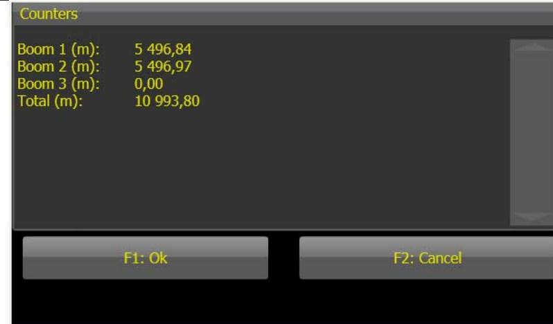
Shows counter values for the drifter and hydraulic pump. Values shown can vary from drill rig to drill rig.
