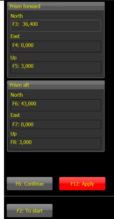
To navigate the drill rig manually using a total station to find the positions of the prisms on the drill rig. Use a prism constant of 46mm. Type the values into the appropriate fields and press F12:Apply.
