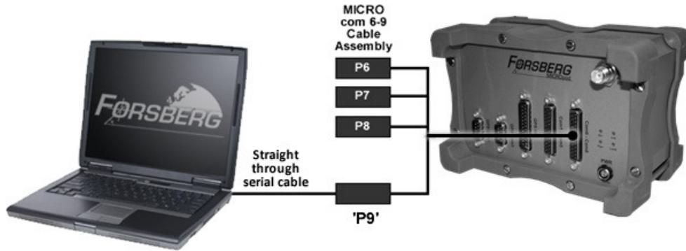
**Figure 9 PC to MICROpod Connection**
