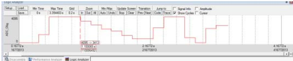
Fig. 13: Simulating the Pot and A/D Conversion using Logic Analyzer
