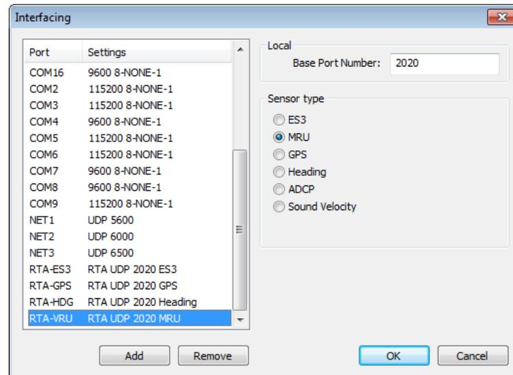
Figure 2-10 Interfacing with RTA port for the VRU
