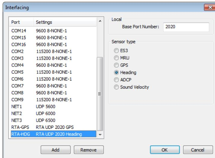
Figure 2-12 Interfacing with RTA port for the compass
