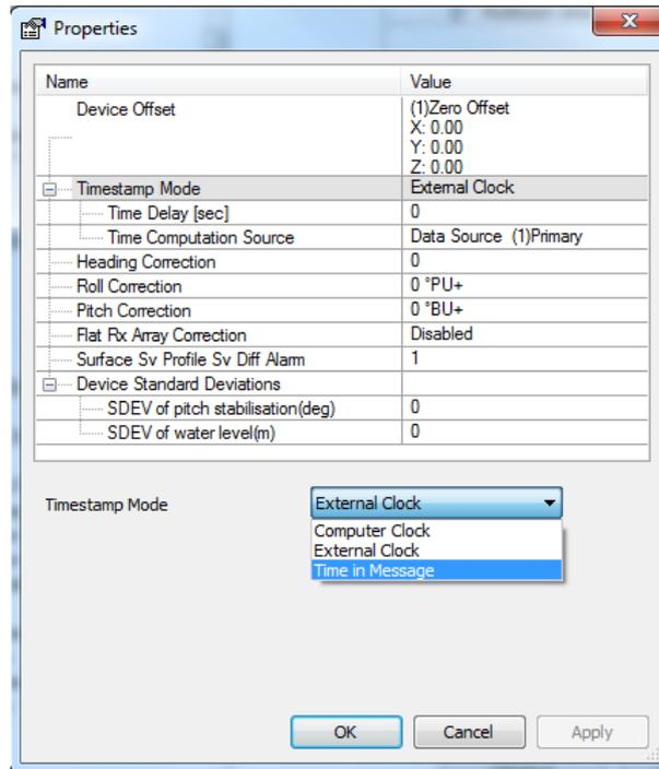
8 Note in this property display you could also select the correct offset for the Multibeam.
