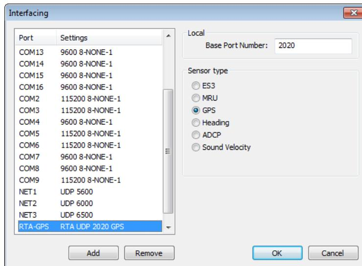
Figure 2-4 Interfacing dialog with the new port for the ZDA message from the RTA box
