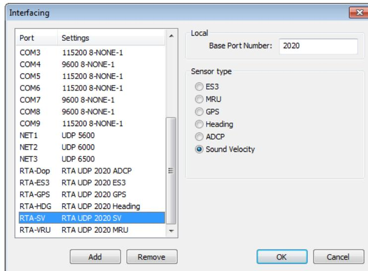
Figure 2-14 Interfacing with RTA port for the sound velocity
