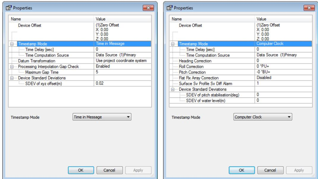
Figure 2-6 Timestamp Mode is Time in Message for the Positioning System (left) and is Computer Clock for the other devices, here the Odom ES3 (right)
