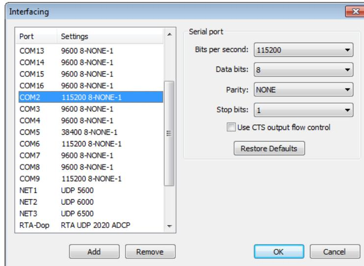
Figure 2-5 Interfacing dialog with the serial port for the 1 PPS pulse
