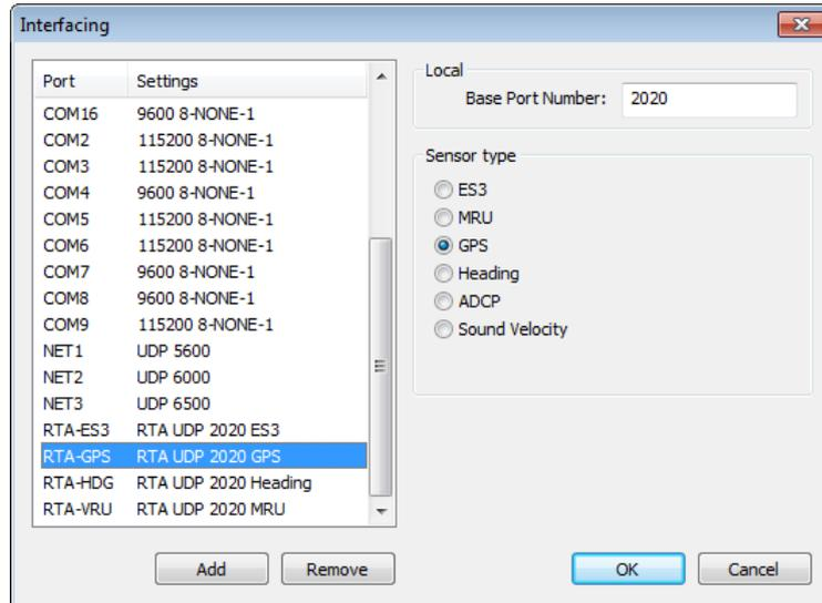
Figure 2-11 Interfacing with RTA port for the positioning system
