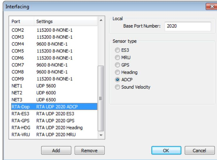
Figure 2-13 Interfacing with RTA port for the doppler
