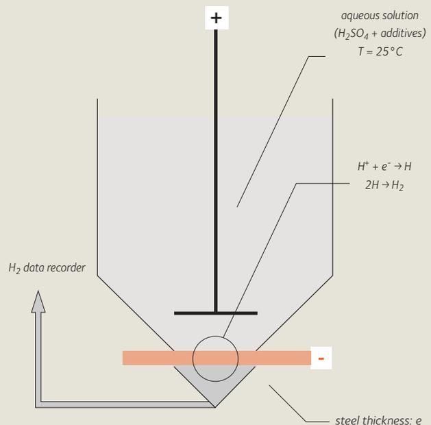
This test can only be used on steel with cavities, i.e. aluminium-killed steel. In the case of IFS, susceptibility to "fish scale" defects is measured by means of an enamelling test in a moist atmosphere or by using a low-adhesive ground-coat enamel (sensitive ground coat).
