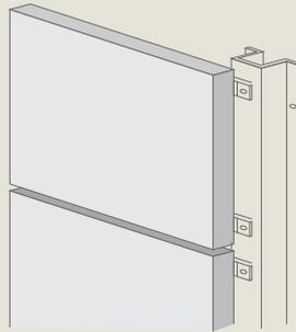
Fixing of flat enamel panels in a tunnel. High-quality stainless steel sub-frame
