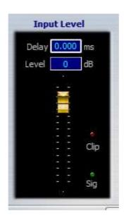
Main delay in ms, meters or feet can be adjusted in this section. The input level is adjusted by the fader control, it provides signal and clipping indicators.
