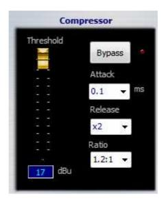
The input compressor has four controls: Attack, Release, Threshold and Ratio. Click on the dropdown list to adjust each parameter. Click the Bypass button to turn it off.
