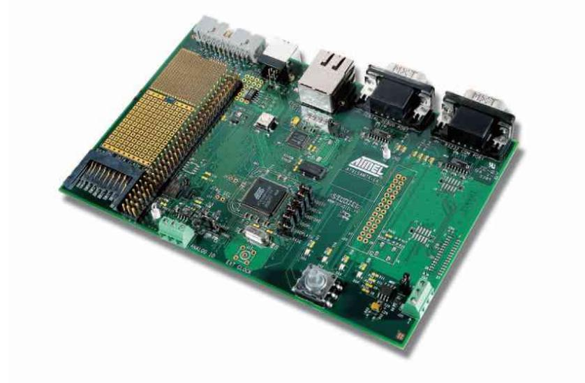
**Figure 10-21.** AT91SAM7X-EK board with AT91SAM7X256.
