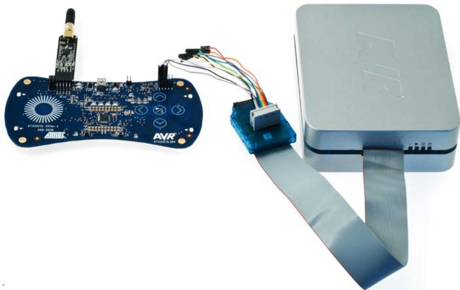
AVR ONE! with AT32UC3L-EK connection details:
