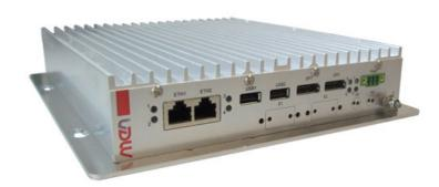
The BC50I is a fanless, maintenance-free box computer that has been designed for independent use or as display computer electronics for use in industrial applications, e.g. for machine control, surveillance or commercial vehicles or robotics.
