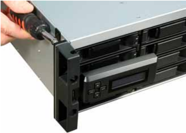
Figure 2. Attach the LCD panel to the VessRAID enclosure
