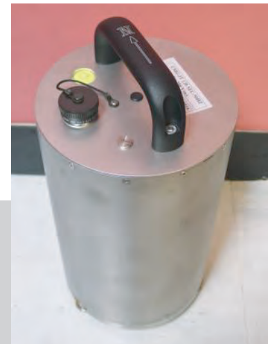
Guralp CMG-3T (or 3T-B borehole) broadband seismometer (120-360 second period)
