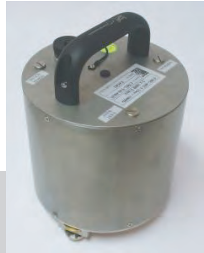
Guralp CMG-40T medium period seismometer (30-60 sec to 50-100Hz)
