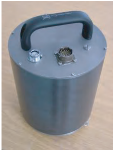
Guralp CMG-3ESP Compact long period seismometer (120 second period)
