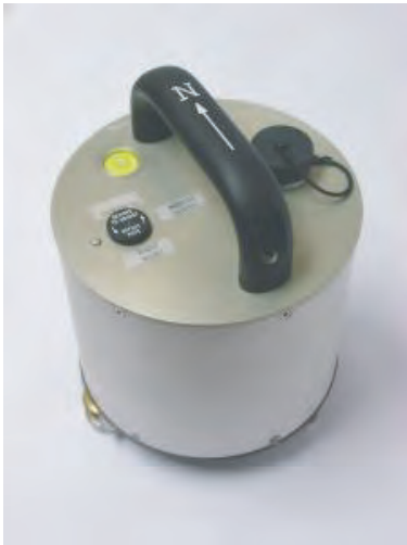
Guralp CMG-6T short period seismometer (1-30 sec to 50-100Hz)
