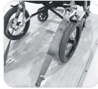
Fitting the rear restraint
