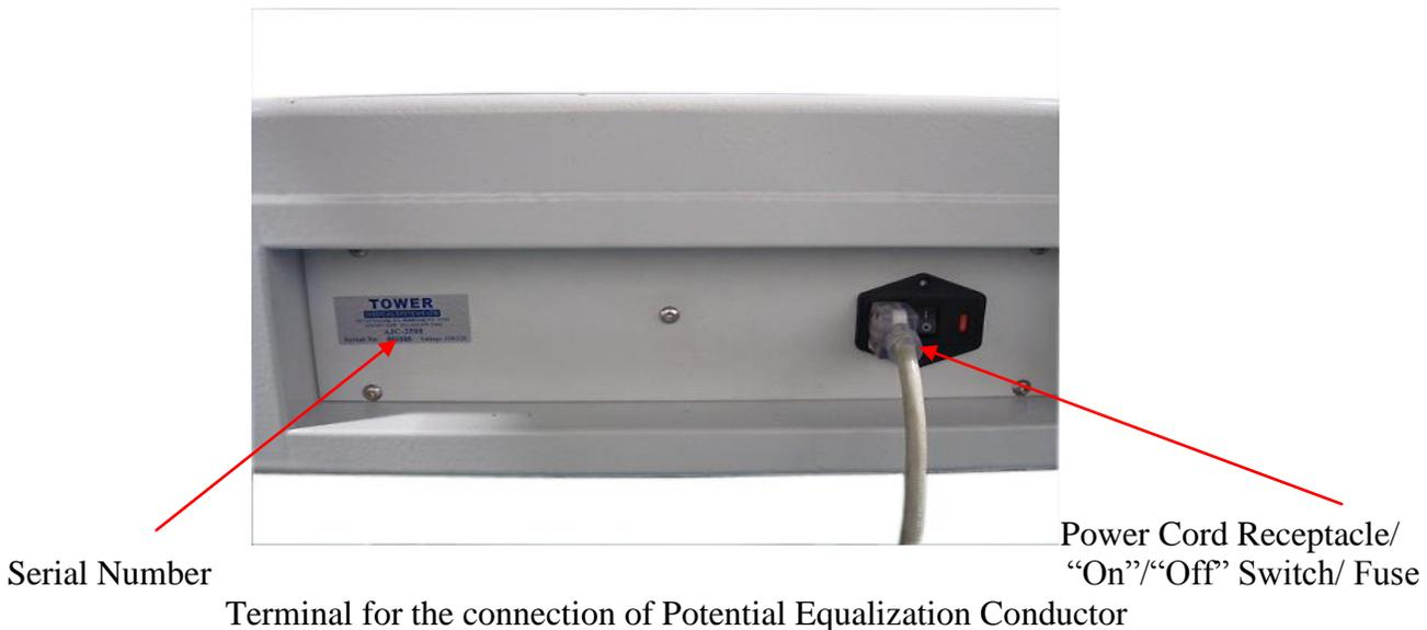
**Figure 2.2-Serial Number/Identification Number**
