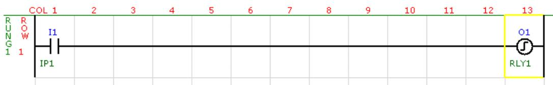
In the following example, when input I1 goes on the output O1 will be reset off. When input I1 is off the output O1 will stay off.
