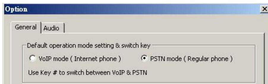
When SkyATA-102 is set in IM Mode and the default operation mode is VOIP, user can press “#” key from phone keypad to switch to PSTN mode, after hearing the familiar PSTN dial tone, user can make regular PSTN calls just as did before. If the default operation mode is PSTN, user just picks up phone and makes regular PSTN calls.
