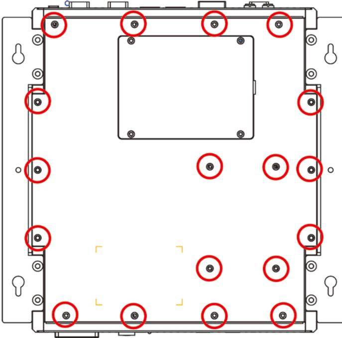
3. Remove the bottom cover. Then, remove the four screws from the storage tray cover.
