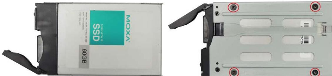
5. Insert the storage device tray into the slot and secure it in place by pushing in the spring-loaded latch.
