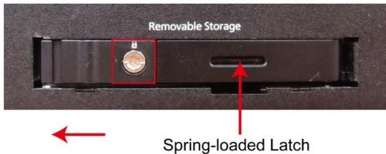
3. Remove the storage device tray from the slot and turn it over.
