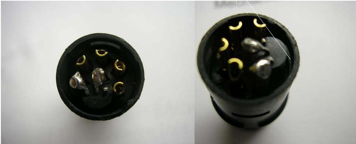
4. Maintain >0.125” clearance between component and connector wall. This is required to allow complete assembly of connector backshell.
