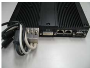
Figure 3.5. Using example of cable clamp
