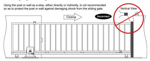
In sake of safety, a positive stop must be mounted on the two end of ground track.
