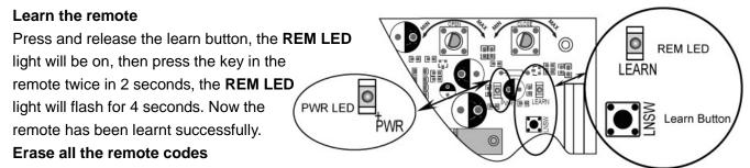
Press and hold the learn button until the REM LED light is off. Now all remote codes have been erased.
