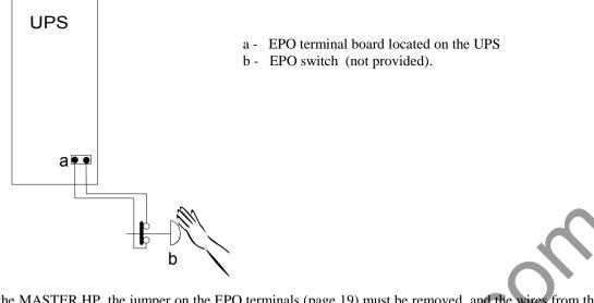
On the MASTER HP, the jumper on the EPO terminals (page 19) must be removed, and the wires from the auxiliary contact of the button must be connected in place of the jumper. The contact must be closed with the button in the rest position and must open when the button is pressed.
