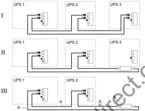
A)UPS parallel cable type RJ45
