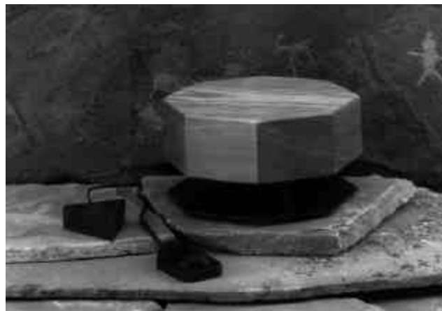
Figure 6. Conference-style FM microphones (photo courtesy of Audio Enhancement).
