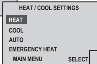
Use the UP or DOWN arrows to highlight HEAT, COOL or AUTO. Press SELECT. The SELECT button will turn on (or off) the desired cycle. You do not have to turn off HEAT to turn on COOL. When HEAT or COOL or AUTO is turned on, all others are automatically shut off. After pressing the SELECT button, the main screen will automatically appear.
