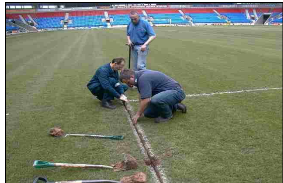
Push sensor to desired depth
