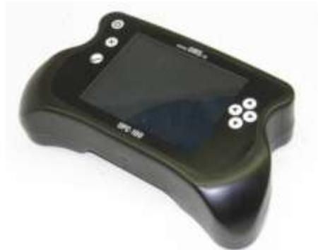
This UPC-100 Handset can be combined with all UMS-developed devices from the UPI series (unless otherwise stated in the specific UPI manual). Depending on the brand of the truck on which the user performs diagnostics/parameterization, a different UPI device must be connected to the UPC-100 Handset.
