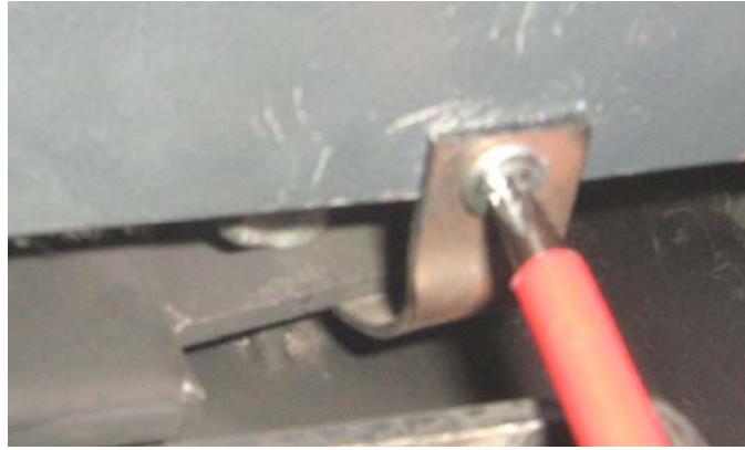
Figure 2.7. Unscrew the front panel fixing screws and remove the panel;
