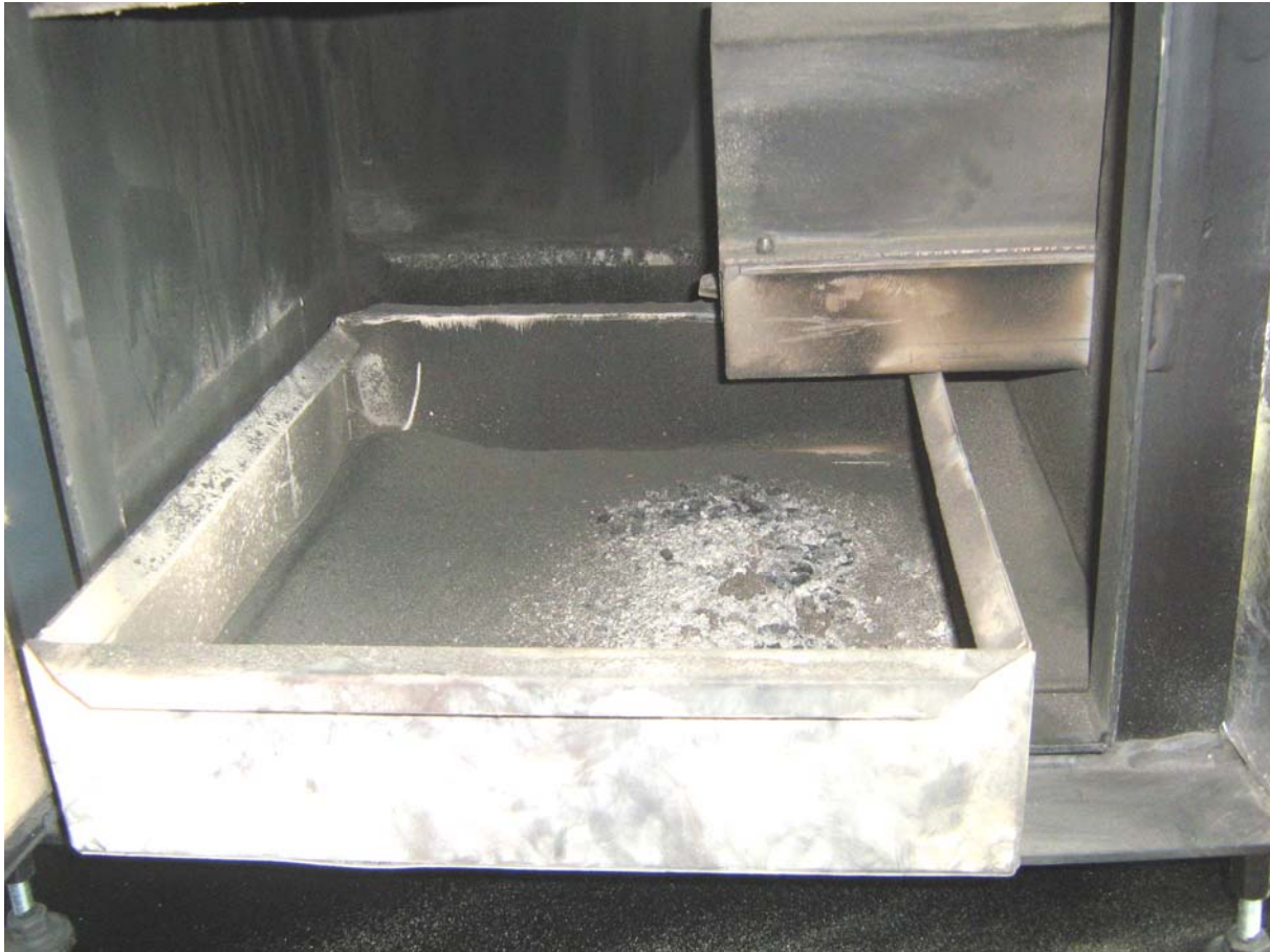
Figure 2.16. Tacking the ash hopper out of the combustion chamber;
