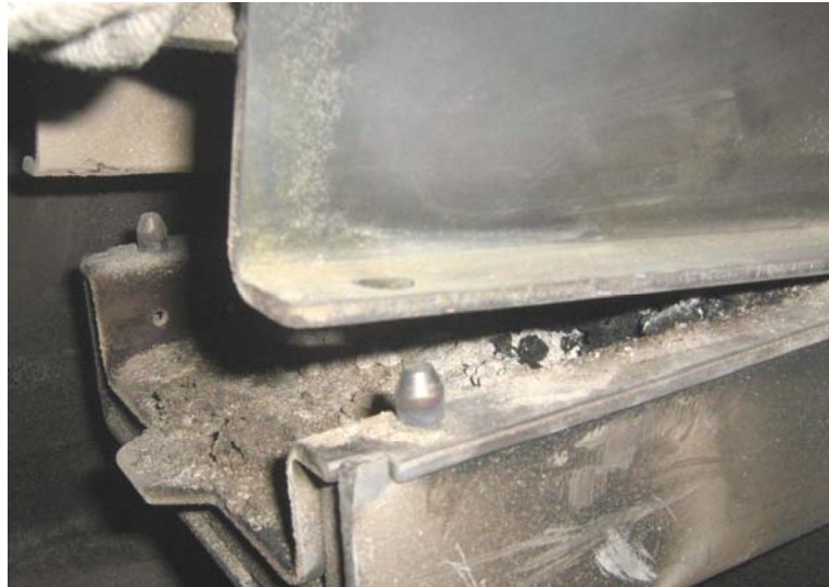
Figure 2.11. Lift of the burner's arc lid;
