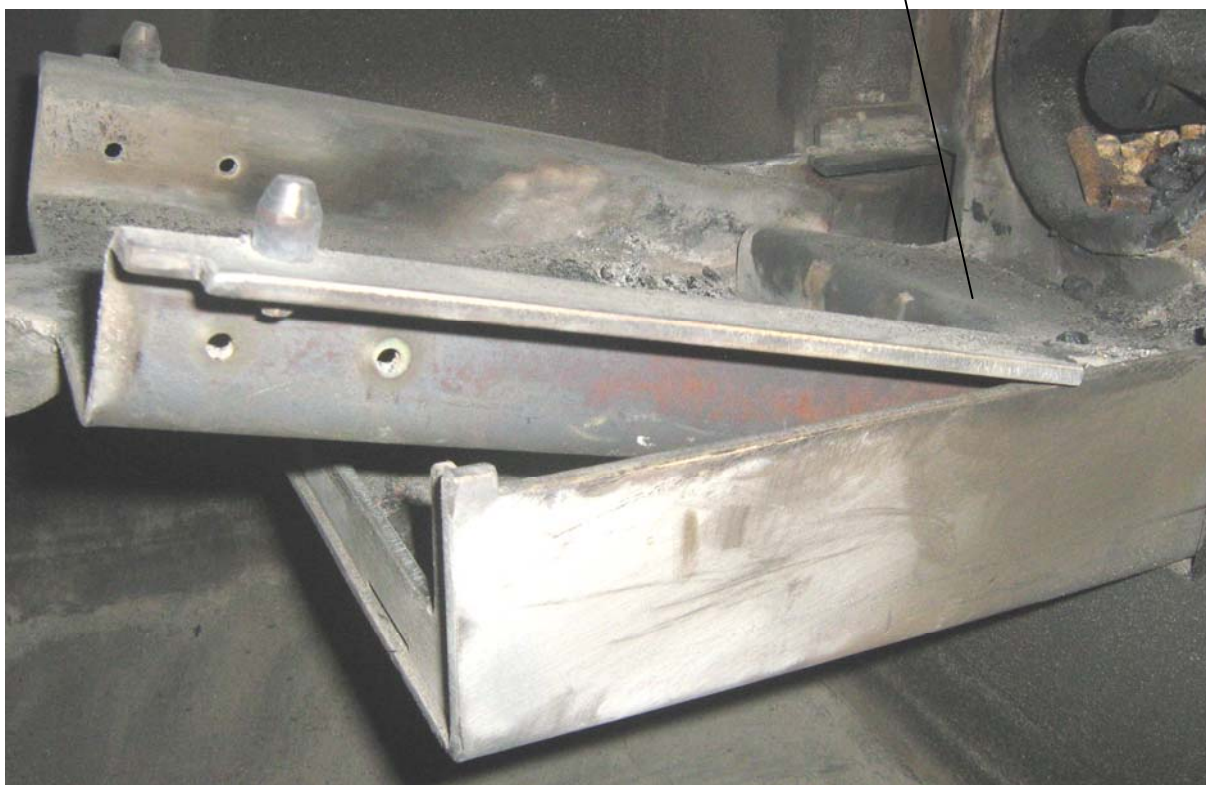
Figure 2.14. Detaching the grate of the specialized burner;
