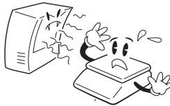
Place the scale on firm and temperature consistent environment.
