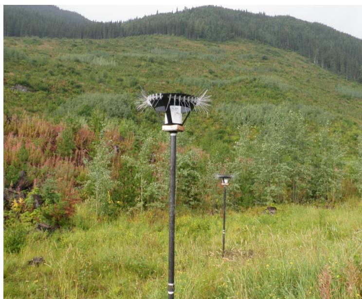
Photo 4.2-5 Dustfall Monitoring Station
