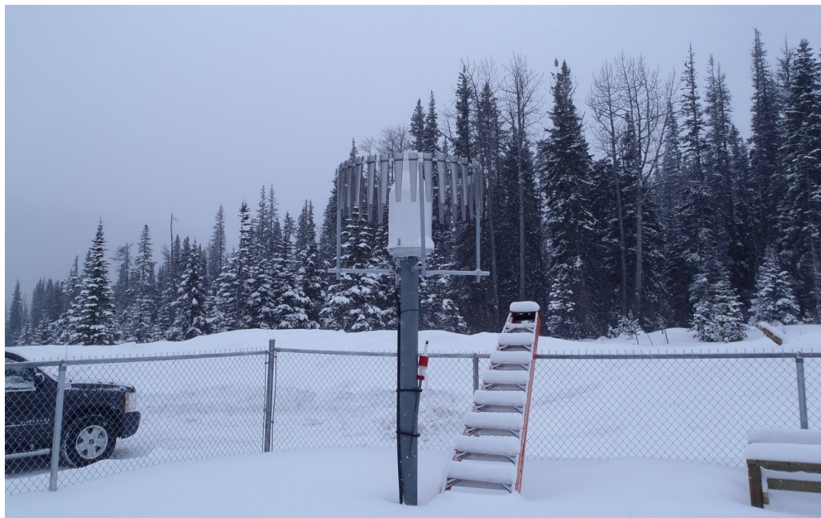
Photo 4.2-3 GEONOR Precipitation Gauge with a Capacity of 1,500 mm
