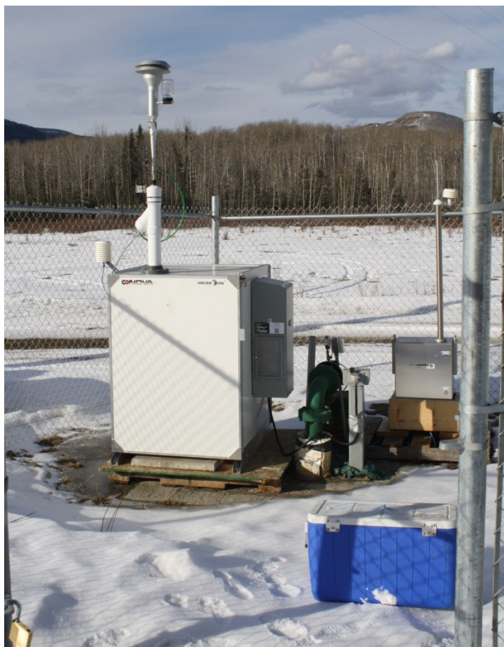
Photo 4.2-4 SHARP and GRIMM PM Monitors at the District of Chetwynd Monitoring Site
