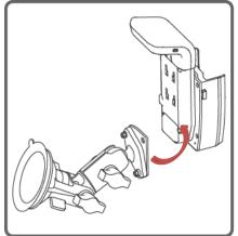
Step 1. First, join the RAM Mount to the joint slot located at the back of the Vehicle Cradle.
