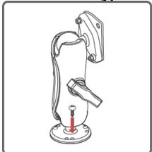
Step 1. First, use screws to fasten the RAM Mount on the dashboard.
