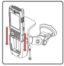
Step 4. Slide PDA into the Vehicle Cradle. It clicks when a PDA is on the right position. After use, press and hold the Release Button to slide out the PDA from the Vehicle Cradle.
