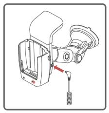
Step 3. Plug in the Cigar Jack cable to Cigar Jack of the vehicle and DC Jack to power connector of the vehicle cradle
