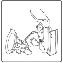
Step 2. Turn the knob from OFF to ON to attach the RAM Mount on the windscreen. Adjust the angle using the fastening knobs of RAM Mount.
