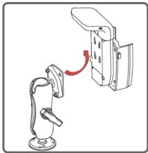
Step 2. Join the RAM Mount to the slot located at back of the Vehicle Cradle. Then, adjust the angle using the fastening knob of the RAM Mount.
