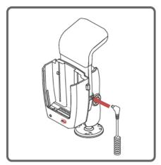
Step 3. Plug in the Cigar Jack cable to Cigar Jack of the vehicle and DC Jack to power connector of vehicle cradle
