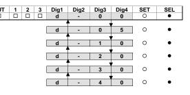
At each pressure of the SEL pushbutton, the different delay levels in ms are visualised in a cyclical manner at the output deactivation and moreover, the relative delay value will be stored When the "d-00" message is visualised the operating mode will be "run", and "rund" in all other cases.
