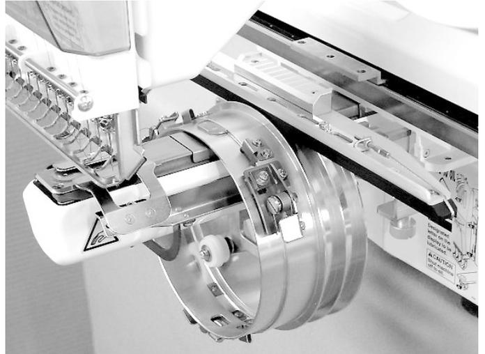
7. Move the cap drive frame in the direction of the arrow, adjust right-and-left mount base to carriage arm and fix them by knob bolts.
