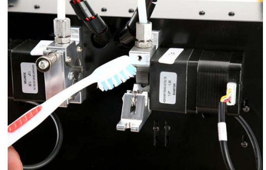
3. Clean small plastic particles with a brush.
