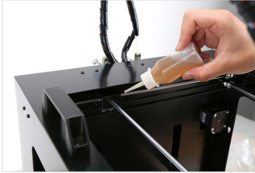
2. Lubricate the X-Y axis and rail guides periodically, no overflow is appropriate.
