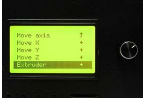
2. Select "Prepare" > "move axis" > "move 1mm" > "move extruder". The feeder gear will start to work.
