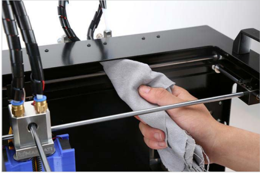
1. Clean the X-Y axis and guides rails.
