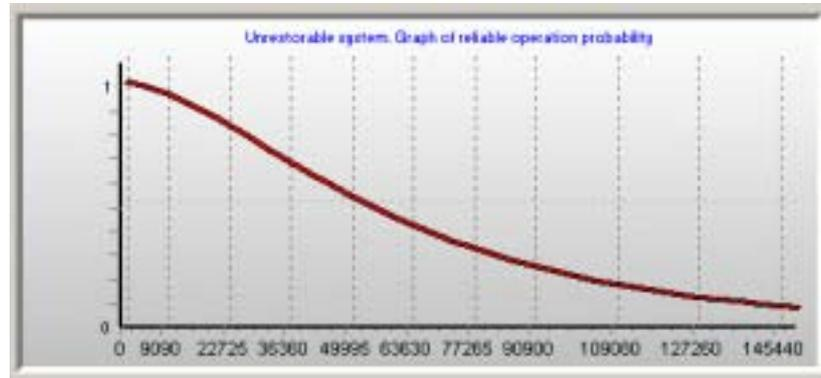
**Fig. 35. The system non-failure operation probability graph**
