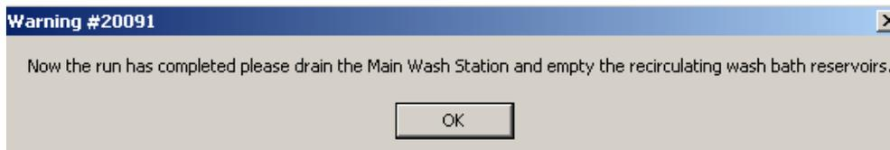
It is recommended to change the wash solutions after every print run and to leave the reservoirs dry if the MicroGrid II will not be used for a while. This is to prevent possible bacterial growth within the reservoirs which may lead to contamination of your samples and damage to the instrument.
