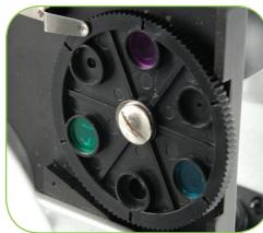
**DIAPHRAGM** – Within the filter wheel are three diameter openings – (1) 1 mm, (3) 3 mm and (6) 6 mm, which limit the amount of light passing through to the specimen. These openings are part of the diaphragm which allows you to change diameter sizes to maximize contrast, brightness, etc. The default setting is "6".
