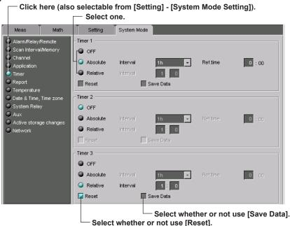
You can set three types of timers. You can have the data saved to a TLOG file or reset the TLOG computation when the specified timeout time elapses.
