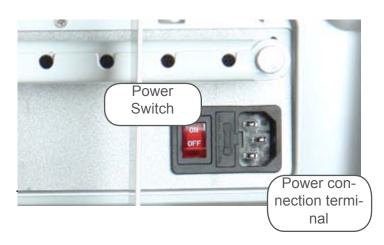
② Turn the sub power switch on the front side of the device ON.
