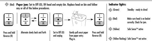
Note: If Safe Sense™ light remains on, you must engage override switch in order to perform above steps.
